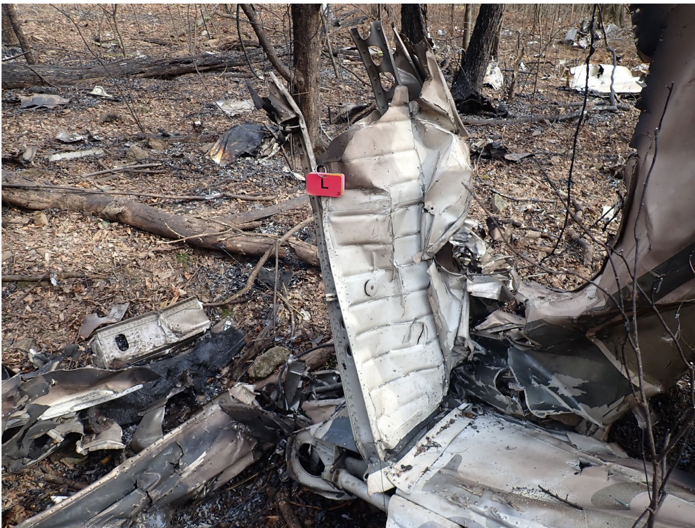
Photograph 4 - View of left elevator and vertical stabilizer.
