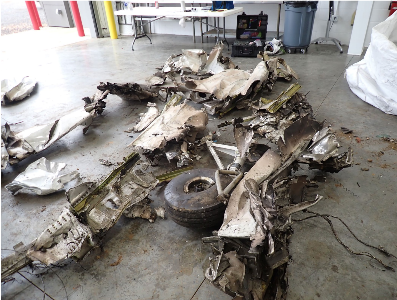
Photograph 7 - View of left wing and landing gear during hangar floor layout.
